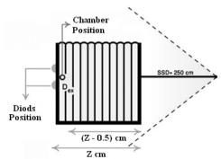
**Figure 3.** Feature of determination of thickness correction factor.
