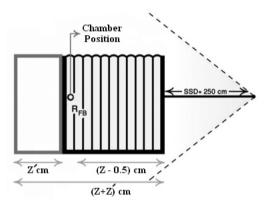
Figure 4. Feature of determination of backscatter correction factor.
