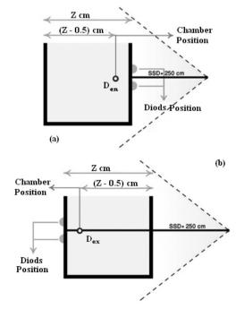
Figure 1. a) Feature of entrance diode calibration, b) feature of exit diode calibration in TBI condition.
