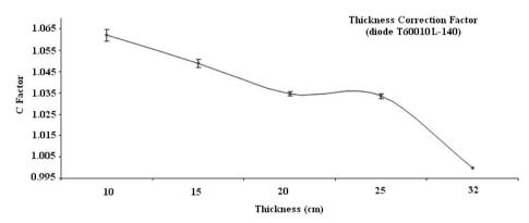
Figure 6. Thickness correction factor as a function of thickness for T60010L-142 diode.
