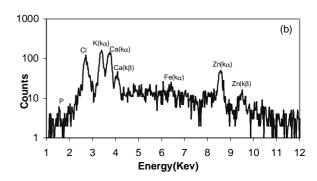
**Figure 1**. Typical spectrum for malignant type of human breast tissue, (a) for low Z elements (without absorber filter) and (b) for high Z elements with  $175\mu$  mylar absorber.
