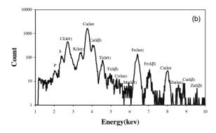
Figure 2. Typical spectrum for benign type of human breast tissue, (a) for low Z elements (without absorber filter) and (b) for high Z elements with 175µ maylar absorber.
