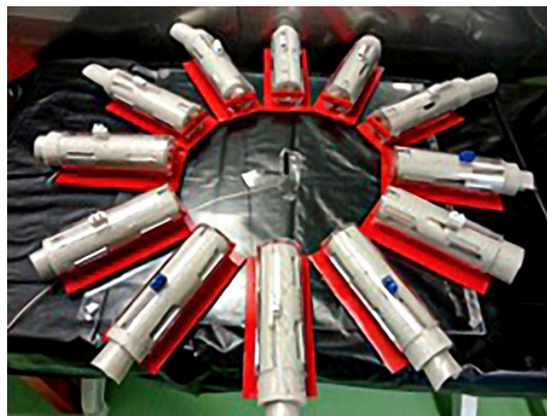
Figure 1. Monopole antenna placement in the carousel exposure setup. All animals were aligned at an equal distance from the central antenna.
