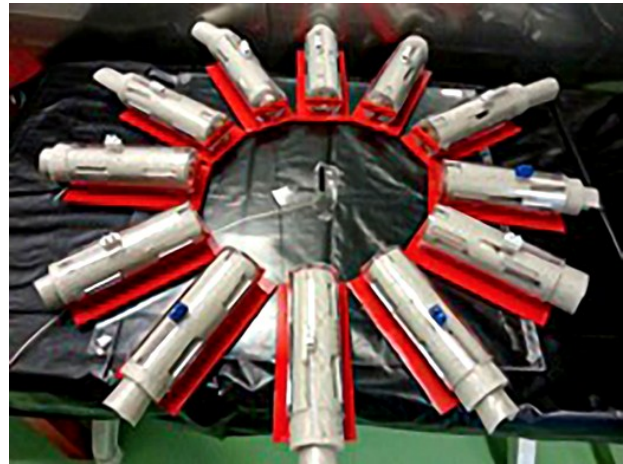
Figure 1. Monopole antenna placement in the carousel exposure setup. All animals were aligned at an equal distance from the central antenna.
