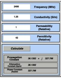
**Figure 2.** Attenuation constant and internal electric field values were obtained by GUI of software.
