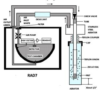
Figure 2. Schematic diagram of Rad 7.
