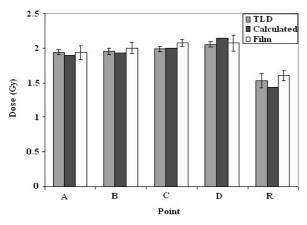
**Figure 4.** Comparison of the mean absorbed dose by TLD and film with planned dose in three-field technique exposed by 9 MV linear accelerators.
