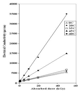
Figure 6. Effect of irradiation temperature on the RIC – absorbed dose dependence of SED (absorbed dose rate = 2.41 kGy/h)
