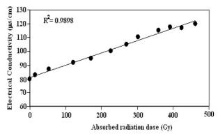
Figure 1. Dose response of SED at low dose range 0-462Gy using 137Cs gamma radiation at 0.035kGy/h.
