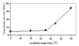
**Figure 7.** Effect of irradiation temperature on the sensitivity ( $\mu$ s.cm<sup>-1</sup>/kGy) of SED (absorbed dose rate = 2.41kGy/h).
