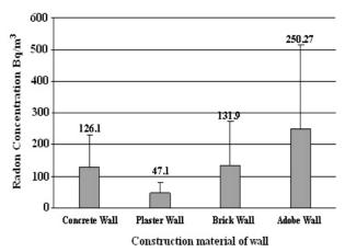
**Figure4.** The wall construction materials of building undergrounds.
