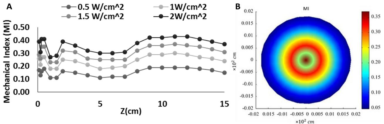
**Figure 2.** The estimation of mechanical index (MI): **A)** The axial mechanical index of a 1MHz frequency transducer in water at 37°C with intensities of 0.50, 1.00, 1.50, and 2.00 W/cm<sup>2</sup> on the z axis in cm; **B)** Radial contour of MI with maximum of 0.39 at a 2 cm distance from the ultrasonic transducer. The color map from blue to red demonstrates an increasing rate of MI.
