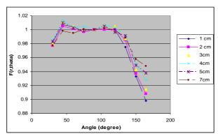
**Figure 4.** Comparison of the anisotropy function at different distances and angles from the source.
