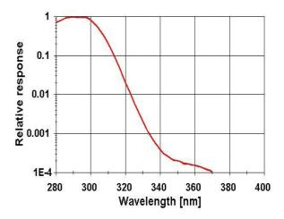
Figure 1. Spectral response of UV-Biometer Model 501.
