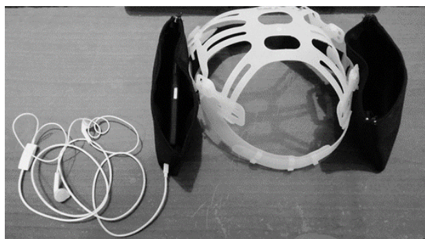
Figure 1. The device used to place a mobile phone on the heads of participants. Connecting the headphones to the mobile phone caused the sound to mute.
