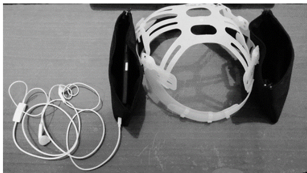
Figure 1. The device used to place a mobile phone on the heads of participants. Connecting the headphones to the mobile phone caused the sound to mute.
