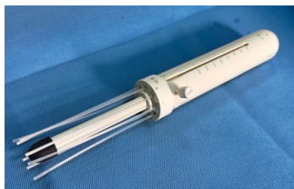
Figure 3. The applicator has nine channels, including one central channel and eight surrounding channels, with a radius of 3.5 cm.
