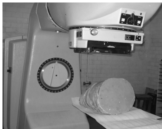
Figure 2. Photograph of heterogeneous phantom in the treatment position with Co-60 machine.
